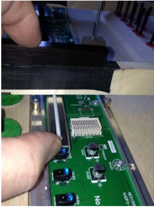
Ill. 7 – Checking sensor strip height
