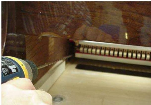
Fig. 21 - Belly rail cable thru hole
