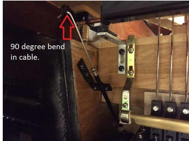
Fig. 22 – Cable bracket secured to rim
