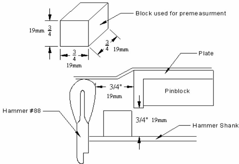
Figure 1 Measuring for clearance
