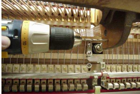
Fig. 17 – Marking location for horn screw      Fig. 18 – Drilling pivot bracket screw hole
