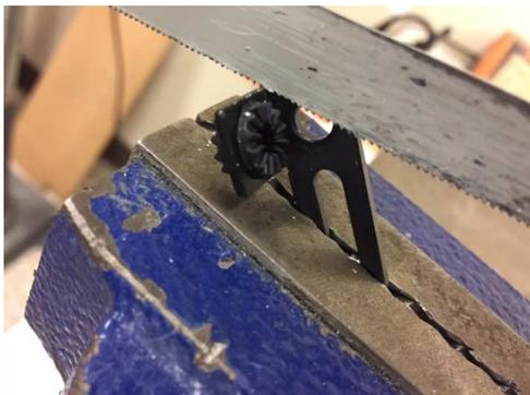
Fig. 15 – Cutting off pivot tang
