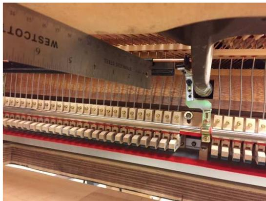
Figure 13 – Mute rail pivot rod height
